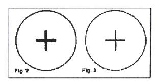
Make sure to take this measure 2 to 3 times to verify that the eyepiece is correctly focused then mark the cylinder and the eyepiece so that in the future this step is easier to perform.
