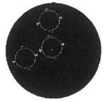
To clear the mires, you will need to adjust the focusing knob (part 7) until the focusing circle is superimposed (above left). Now we lock the keratometer into place with the locking knob (part 8).
